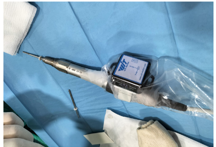
Figure 2. Inclinometer integrated into the surgical motor.
