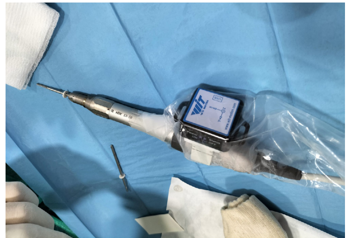
Figure 2. Inclinometer integrated into the surgical motor.
