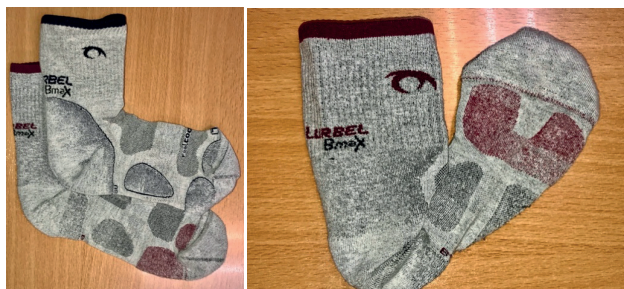
Figure 2. Left; control sock (gray threads) and experimental (red threads). Right, detail of the central discharge integrated in the experimental sock.
